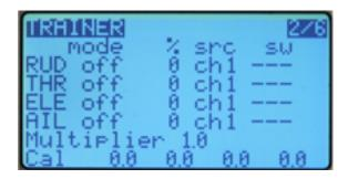
This menu allows the PPMin (trainer) inputs to be configured. It enables the RAW PPM inputs to be selected to replace the sticks for training purposes. The student transmitter does not need to have the same model setup as the instructor. All the mixes on the instructors Tx will be applied to the student inputs. If, for example, you have expo on your sticks, this will be applied to the raw trainer inputs when they are selected.
