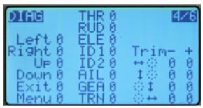
This menu will help you visualize the current state of the trims, keys and physical switches. Each Key/Switch/Trim is represented. When pressing a key or switch they are highlighted.
