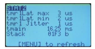
The second shows general timing of the Tx. The value "tmain" shows how long the math takes. This will increase as you add more mixers. It can be very large sometimes depending on eeprom writes. The Stack value shows the unused space, in hexadecimal, between the end of used Ram memory and the lowest point the stack has reached. You can reset the timers by pressing [MENU].
