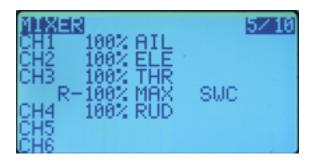
What this is telling you is that the rudder stick's input is being routed with a weight of 100% to CH4. For the elevator CH2, throttle CH3 and aileron CH1.
