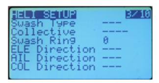
This screen is specifically designed to help you set up a CCPM heli.
