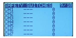
Safety switches allow you to select a switch and have it write a value for a channel that will overwrite any other value.
